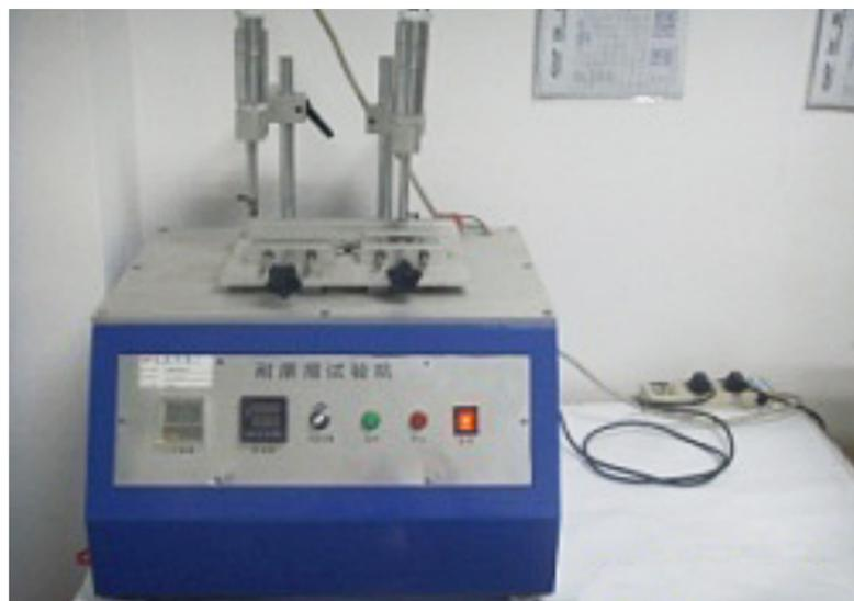
Rub-resistance test for colour fading
